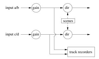
Designing the signal flow in this way is pretty clever as it allows for fading in or out the live inputs, irrespective of the sampling process. I can thus sample without hearing the inputs, or vice versa or any combination.
